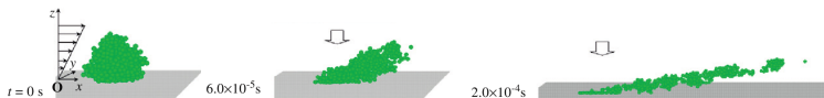
Figure : Snapshots of particle reentrainment from an initially nearly spherical cluster exposed to shear flow (from Iimura et al., Chem Eng Sci, 2009)
