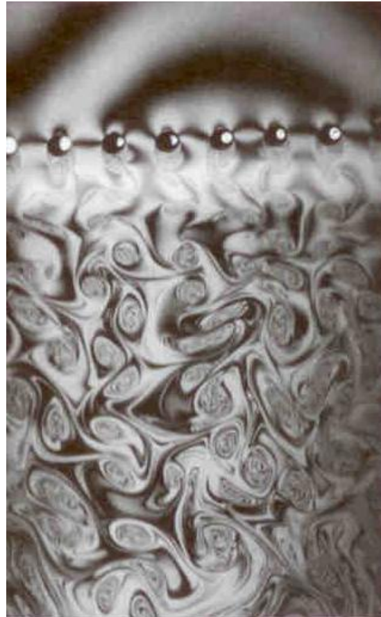
flow through array of rods
