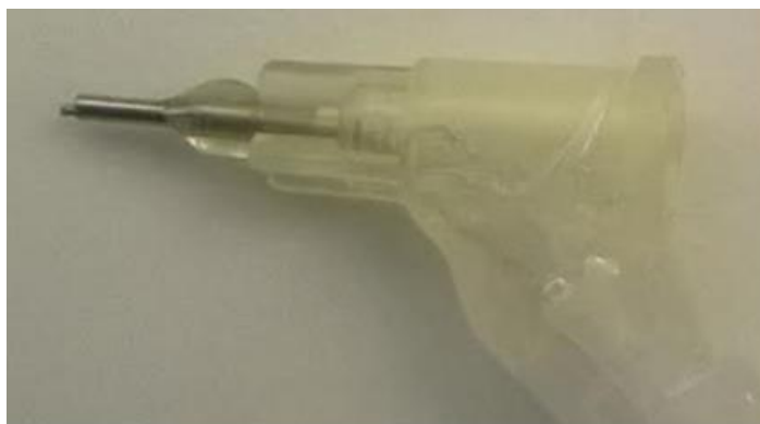
Fig. A5.4. Handmade nozzle, designed and manufactured at IPPT PAN.
