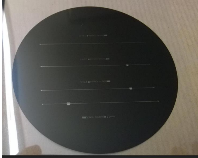
Fig. A6.1. Photography of a mask. The transparent areas of the mask presented the shape of future microchannel structures, through which the UV light during exposure was curing Su-8.
