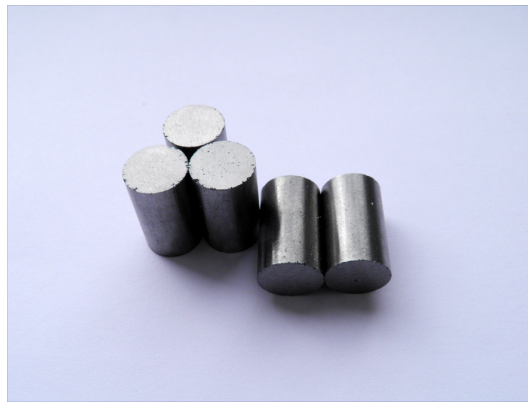
Figure 3.6. Sintered NiAl/Al 2 O 3 specimens
