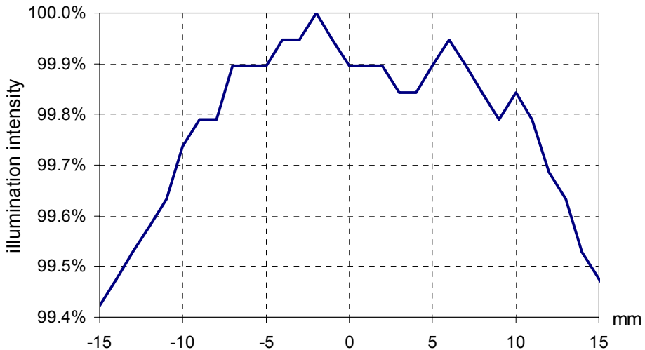
Fig. 5.3 Typical measurement of the illumination uniformity of the CCD sensor (measured radial from the centre and plotted as normalised intensity).
