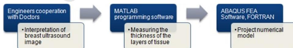
**Fig. 1 – The methodology of breast numerical model development.**
