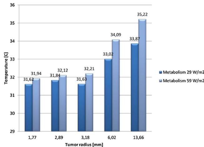
**Fig. 10** – The minimum temperature on the surface of the breast for five selected numerical models. The parameter used in the simulation: the heat transfer coefficient equal to 10 W/mK. The simulation takes into account the type of cancer. The benign cancer was described by 29,000.00 W/m<sup>2</sup> of metabolic heat production and malignant by 58,000.00 W/m<sup>2</sup>.
