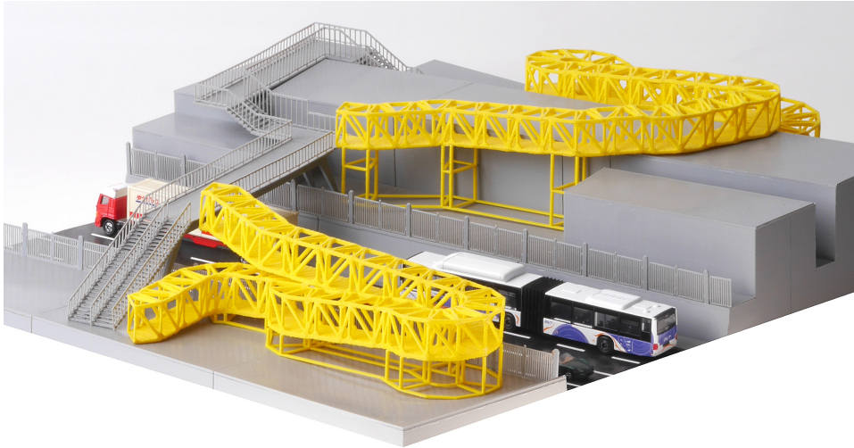
FIG. 1. Photograph of a physical scale model of retrofitting an existing overpass with Truss-Z.
