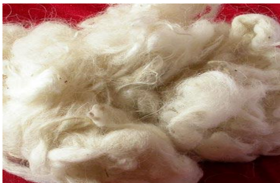
Fig. 1: Sheep wool used to reinforce mortars.
