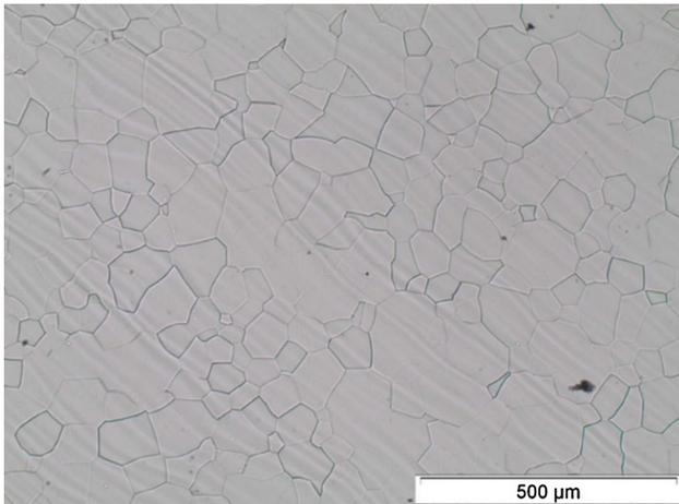
**Fig. 1** Optical microscope image of Gum Metal
