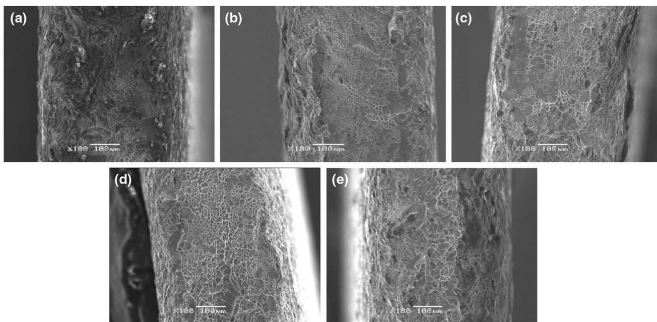
**Fig. 17** SEM fractographs of Gum Metal subjected to tension at strain rates of **a**  $10^{-5} \text{ s}^{-1}$ , **b**  $10^{-4} \text{ s}^{-1}$ , **c**  $10^{-3} \text{ s}^{-1}$ , **d**  $10^{-2} \text{ s}^{-1}$ , **e**  $10^{-1} \text{ s}^{-1}$
