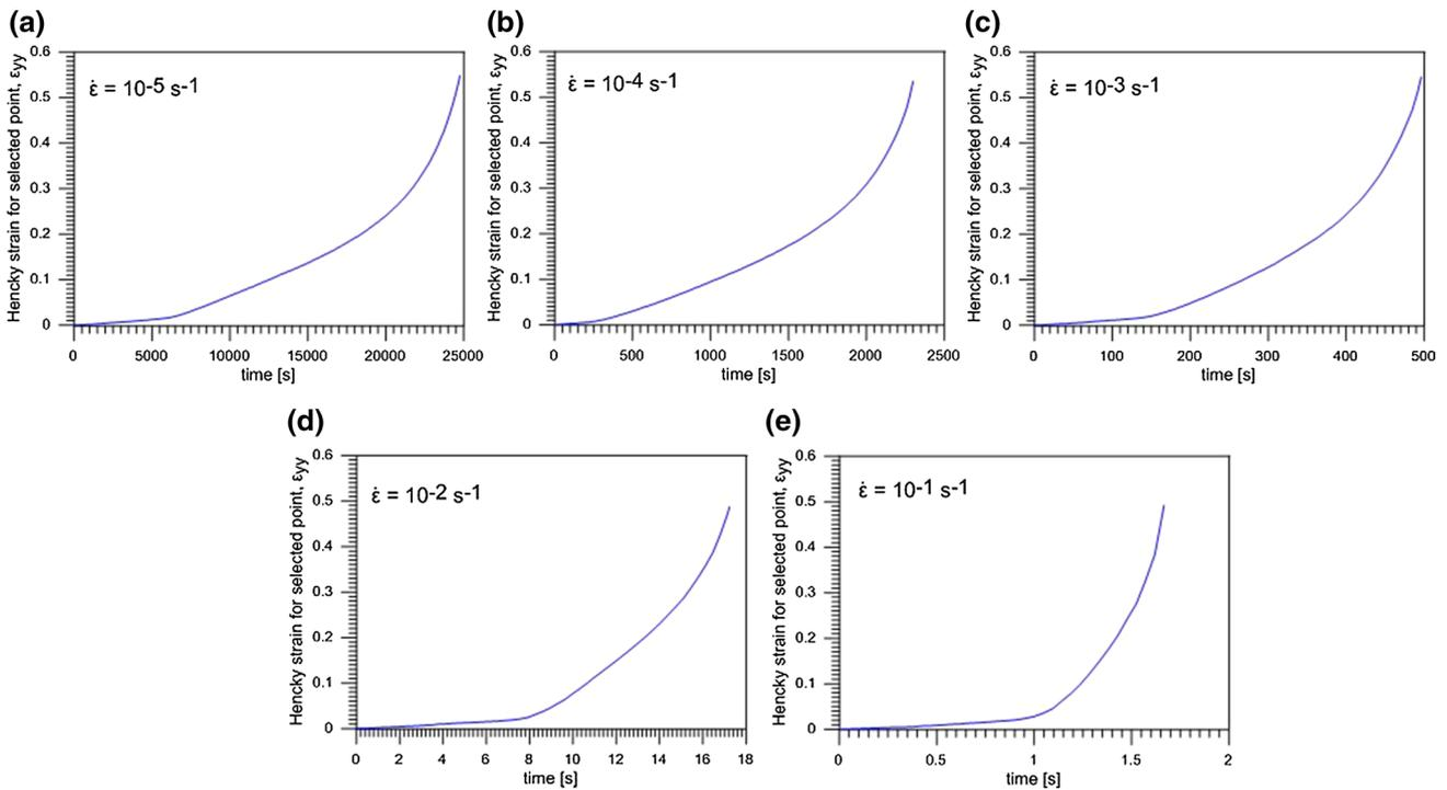
**Fig. 13** Hencky strain  $\epsilon_{yy}$  versus time curves for selected points of Gum Metal under tension at strain rates of **a**  $10^{-5} \text{ s}^{-1}$ ; **b**  $10^{-4} \text{ s}^{-1}$ ; **c**  $10^{-3} \text{ s}^{-1}$ ; **d**  $10^{-2} \text{ s}^{-1}$ ; **e**  $10^{-1} \text{ s}^{-1}$
