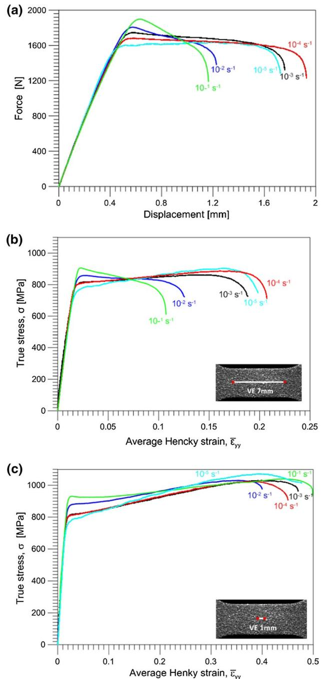
**Fig. 8** Comparison of the mechanical characteristics of Gum Metal subjected to tension until rupture at strain rates:  $10^{-5} \text{ s}^{-1}$ ,  $10^{-4} \text{ s}^{-1}$ ,  $10^{-3} \text{ s}^{-1}$ ,  $10^{-2} \text{ s}^{-1}$  and  $10^{-1} \text{ s}^{-1}$ : **a** force versus displacement and true stress versus true strain curves for **b** VE 7 mm, **c** VE 1 mm
