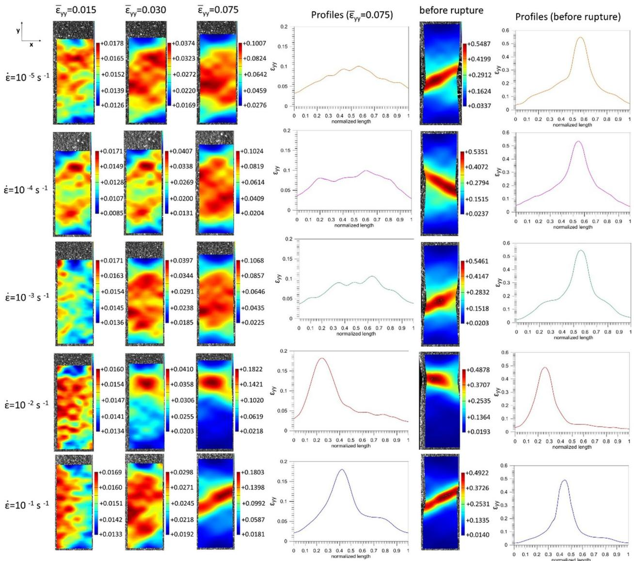
**Fig. 12** Development of Hencky strain  $\epsilon_{yy}$  distributions of Gum Metal subjected to tension until rupture at strain rates  $10^{-5} \text{ s}^{-1}$ ,  $10^{-4} \text{ s}^{-1}$ ,  $10^{-3} \text{ s}^{-1}$ ,  $10^{-2} \text{ s}^{-1}$  and  $10^{-1} \text{ s}^{-1}$  and selected strain  $\epsilon_{yy}$  profiles
