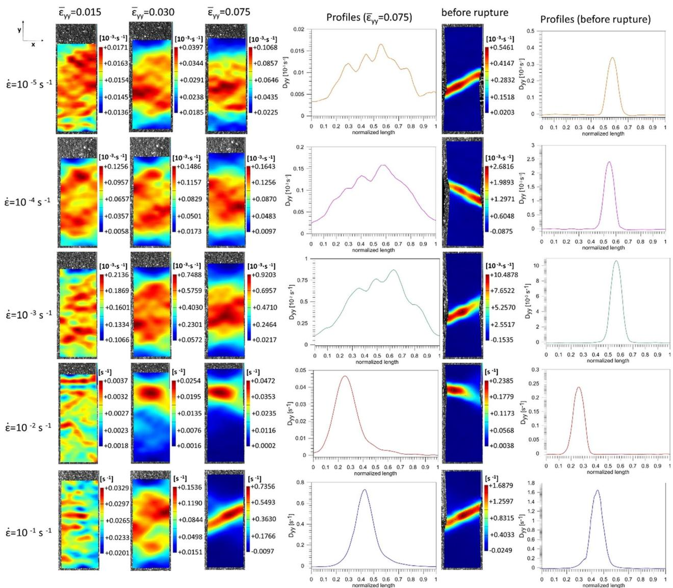
**Fig. 15** Development of the rate of deformation tensor  $D_{yy}$  distributions at strain rates  $10^{-5} \text{ s}^{-1}$ ,  $10^{-4} \text{ s}^{-1}$ ,  $10^{-3} \text{ s}^{-1}$ ,  $10^{-2} \text{ s}^{-1}$  and  $10^{-1} \text{ s}^{-1}$  and selected strain  $D_{yy}$  profiles
