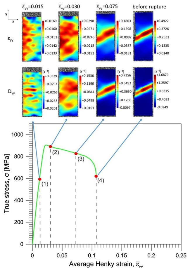
**Fig. 11** Distributions of the Hencky strain  $\varepsilon_{yy}$  and rate of deformation tensor  $D_{yy}$  components of Gum Metal under tension at strain rate of  $10^{-1} \text{ s}^{-1}$  at four stages of loading denoted by (1), (2), (3) and (4)
