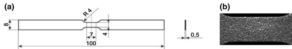
**Fig. 7** Experimental setup used for the investigation of Gum Metal under tension at various strain rates: a diagram, b photograph
