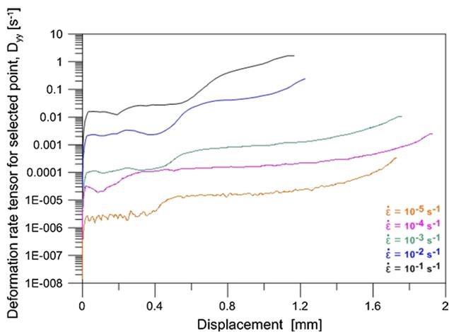
**Fig. 16** Deformation rate tensor  $D_{yy}$  versus displacement curves for selected points of Gum Metal under tension at five strain rates:  $10^{-5} \text{ s}^{-1}$ ;  $10^{-4} \text{ s}^{-1}$ ,  $10^{-3} \text{ s}^{-1}$ ,  $10^{-2} \text{ s}^{-1}$  and  $10^{-1} \text{ s}^{-1}$
