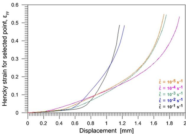
**Fig. 14** Hencky strain  $\epsilon_{yy}$  versus crosshead displacement curves for selected points of Gum Metal under tension at five strain rates:  $10^{-5} \text{ s}^{-1}$ ,  $10^{-4} \text{ s}^{-1}$ ,  $10^{-3} \text{ s}^{-1}$ ,  $10^{-2} \text{ s}^{-1}$  and  $10^{-1} \text{ s}^{-1}$
