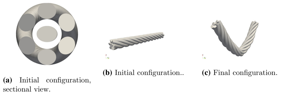
Fig. 19 Example 3: reference and final configurations of the structure. The discontinuous surface of the strings of BFEs, that is improper for contact treatment, is shown. On the right, one can observe the effect of the rotations applied to the sections at the ends of the rope
