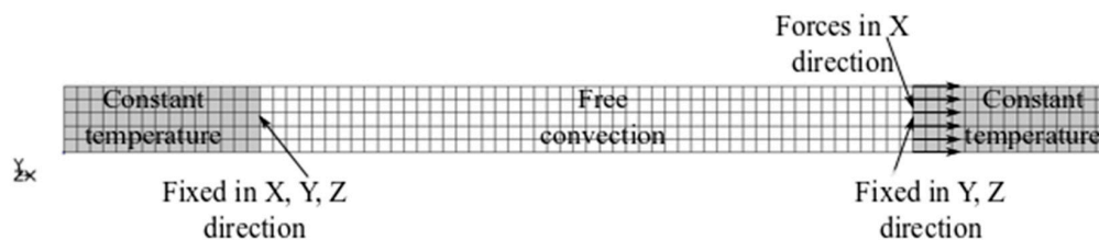
Figure 4. A mesh for the finite element model (FEM) of the SMA specimen showing loading and boundary conditions.
