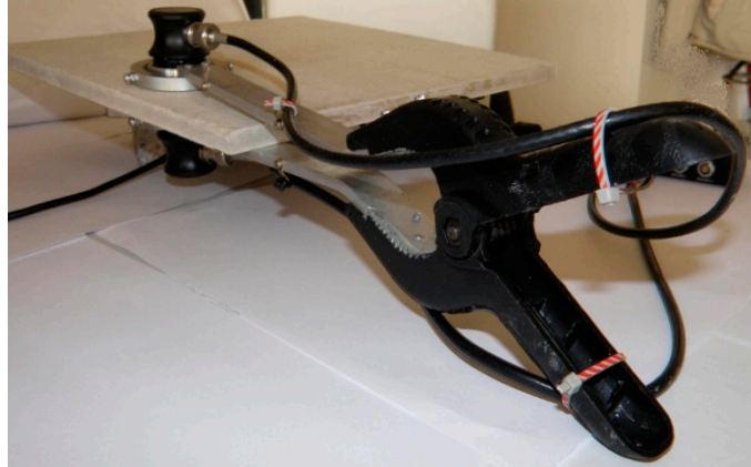
Figure 3. Detailed view of the custom-designed holder for correct coupling between the ultrasonic transducers and both sides of the rough surface board.
