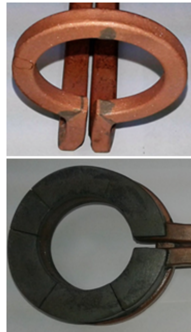
Fig. 8. MF inductor (up) and HF inductor – sprayer (down)
