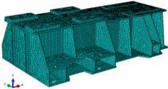
Fig. 4. The 3D FEM model of the machine foundation frame.
