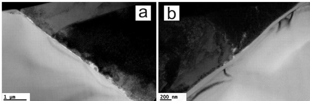
Fig. 7. TEM images of copper-silicon carbide interface.
