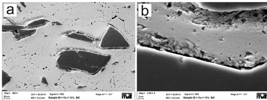
Fig. 3. SEM image of the hot-pressed Cu-15SiC composite structure (a) and ceramic-metal interface (b).
