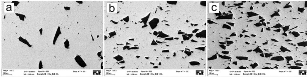
Fig. 4. SEM image of the Cu-SiC composite materials obtained by spark plasma sintering.
