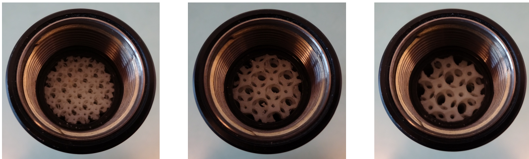
Figure 7: 3D-printed samples of periodic foam (with porosity 83% and various sizes of periodic cell, namely: 5 mm, 8 mm, and 10 mm) inside the impedance tube with diameter 29 mm.
