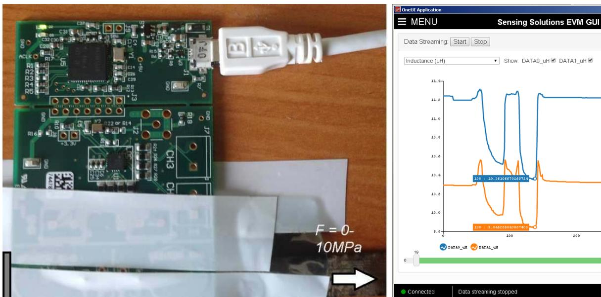
**Fig. 9.** Recording of stress changes in the metallic glass foil
