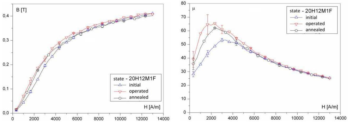
**Fig. 6.** Comparison of changes in steels' operational parameters
