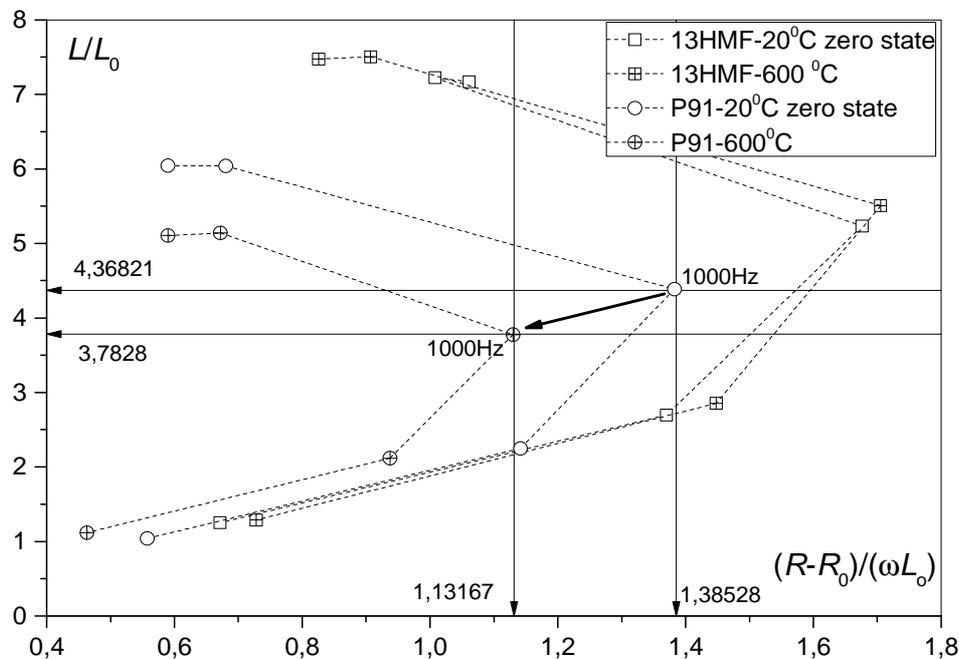
**Fig 7.** Comparison of changes in normalized impedance components, for two types of steel used in power engineering
