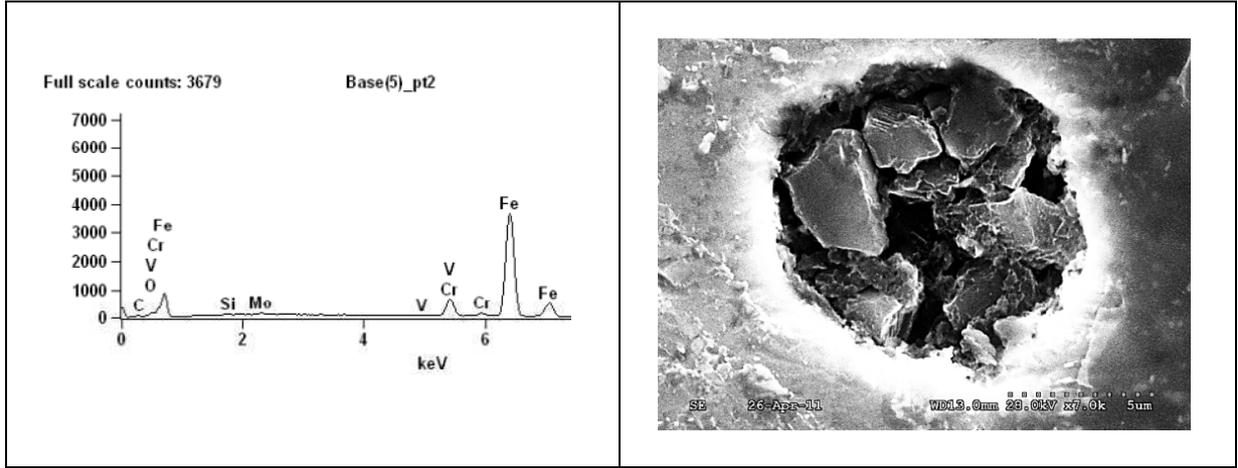
**Fig. 4.** Images and composition of non-metallic inclusions of the input material, before and after mechanical loading at the MTS servo hydraulic machine
