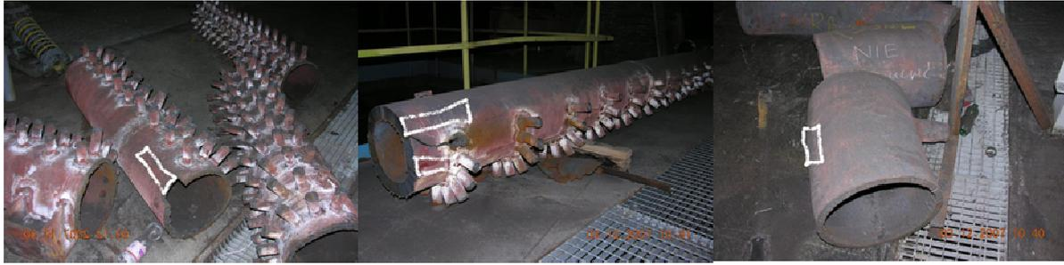
**Fig. 1.** Fragments of power industry installations, locations where samples were obtained are shown; from the left: inlet chamber 15HM, inlet chamber 20H12M1F, knees 13HMF
