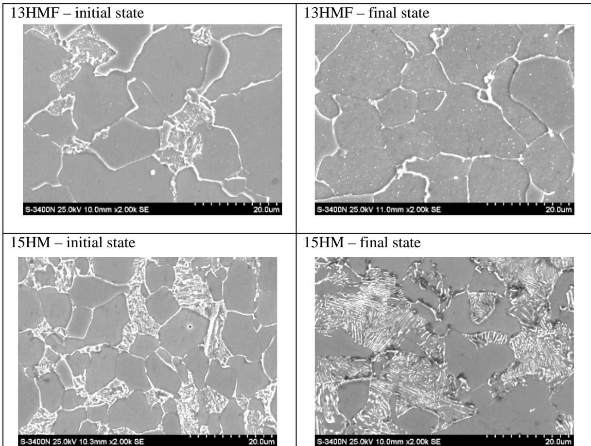
**Fig. 2.** Comparison of changes in steel micro structures for 13HMF and 15HM steels
