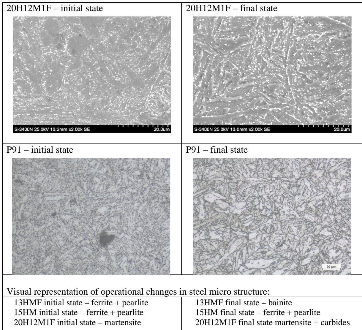
**Fig. 3.** Comparison of changes in steel micro structures for 20H12M1F and P91 steels
