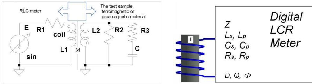
**Fig. 5.** Model of the measurement circuit [1]
