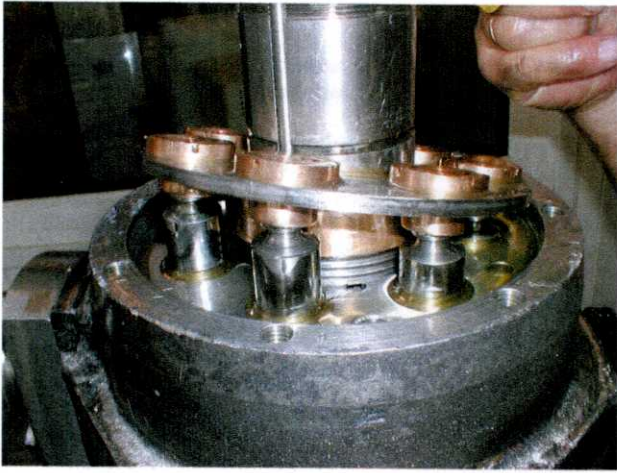
Fig. 1 Swash plate on a novel piston pump with piston slippers—part of the PWK axial piston pump
