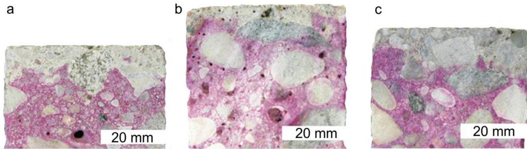
Fig. 6. The carbonation depth measured with the phenolphthalein solution: (a) A-1; (b) B-2; (c) C-2 (the scale bar is shown).
