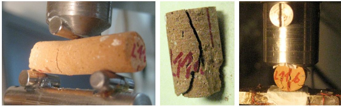
Figure 6: Micro-core L11 after testing using CoDiT method: three-point bending (left), uniaxial compression (center) and diametral compression (right).
