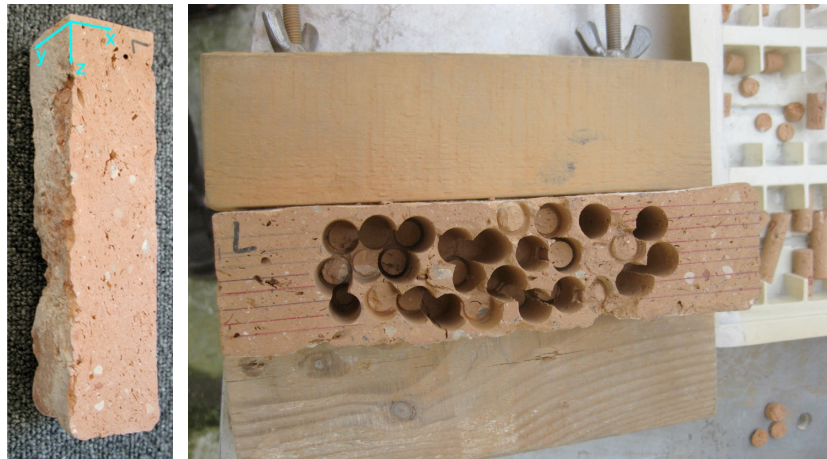
Figure 4: Sample of the brick from Puerta de Burgos with sample coordinate system (left) and drilled micro-core specimens (right).
