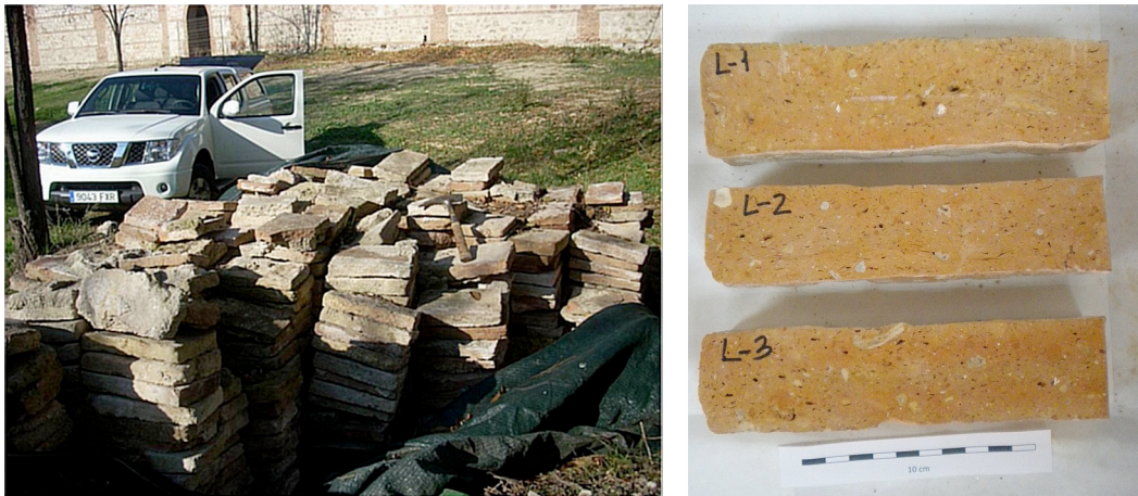
Figure 3: Stockpile of bricks from the 2005's collapse of the structure, left, and bricks sampled (right).
