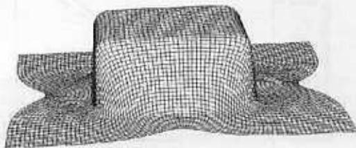
Figure 2. Deformation of the square blank at the punch stroke 40 mm for the cup deep drawing of AISI 4330 steel with application of ABAQUS/EXPLICIT for modified Burzyński yield condition and isotropic hardening law for the punch stroke 40 mm of AISI 4330 steel.
