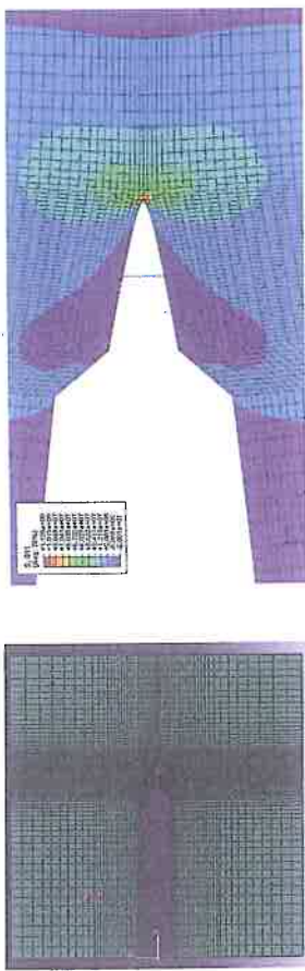
Figure 7. Vertical stress distribution (numerical solution by ABAQUS)
