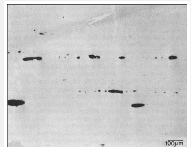
Fig. 15. Spalling by ductile void formation in nickel (after Shockey, Seaman and Curran 1973)
