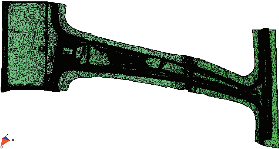
Fig. 2. Geometrical description of final piece (195 079 triangular facets)
