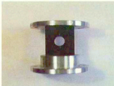
FIG. 3. Complex stress-state specimen.
