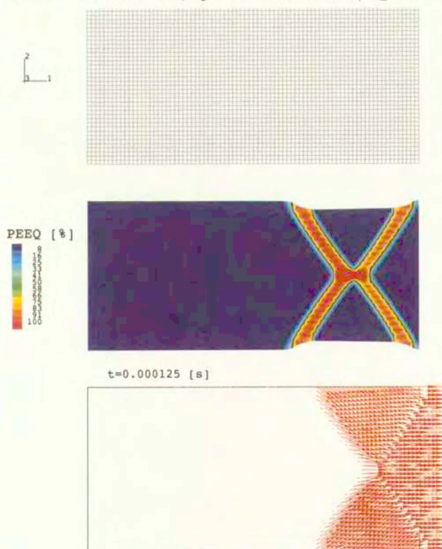
FIG. 1. Mesh, plastic equivalent strain distribution and vector plot of velocity for 2D model.
