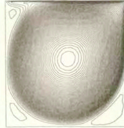
(b) Gradient based procedure, Nodes: 1034, Elements: 1962
