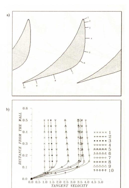
Fig. 5. The averaged boundary layer velocity field distribution calculated at indicated positions.
