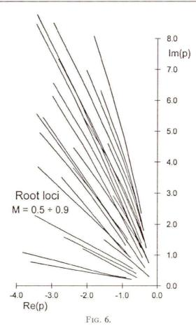
It has been found in the example of a rectangular wing, but also for other surface configurations, that the calculated roots of Eq. (3.5) were always simple roots only.
