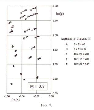
and a large number of aerodynamic elements is required at the discretization. It follows, that the number and distribution of latent roots do not depend on the size of matrix [K(M, p)] within the limits of accuracy of the used method.
