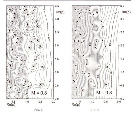
number grows rapidly only in the vicinity of each root. In a very small region ( $|\Delta p| < 10^{-8}$ ), the determinant of the matrix decreases usually by a factor about  $10^{-10}$ , although its value may be still very large. This is shown in the Fig. 4, where the contour lines correspond to constant values of  $\log_{10} |\det[K(M,p)]|$ .
