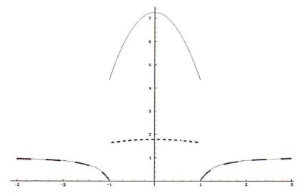
FIG. 2. Dimensionless velocity (as referred to  $v_{\infty}$ ) at the flow symmetry axis as a function of the dimensionless z-coordinate (as referred to R) under the same assumptions about  $\varepsilon_{\eta}$  and  $\varepsilon_{\varrho}$  as in the case of Fig. 1 in the Euler (solid line) and Stokes (dashed line) approximations.
