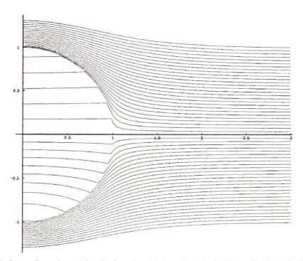
FIG. 1. Streamlines pictures for the flow through the sphere in the Euler (the lower half) and Stokes (the upper half) approximations under the assumptions:  $\varepsilon_{\eta} = \sqrt{\varepsilon_{\varrho}}$ ,  $\varepsilon_{\varrho} = 2.5 \times 10^{-2}$ .
