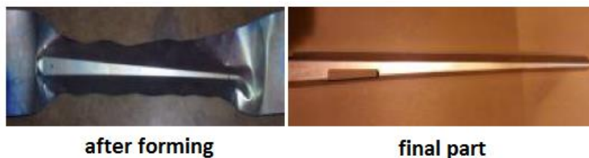
Figure 2-21. Example of an industrial part formed by electric resistance method (Ozturk et al. 2016).
