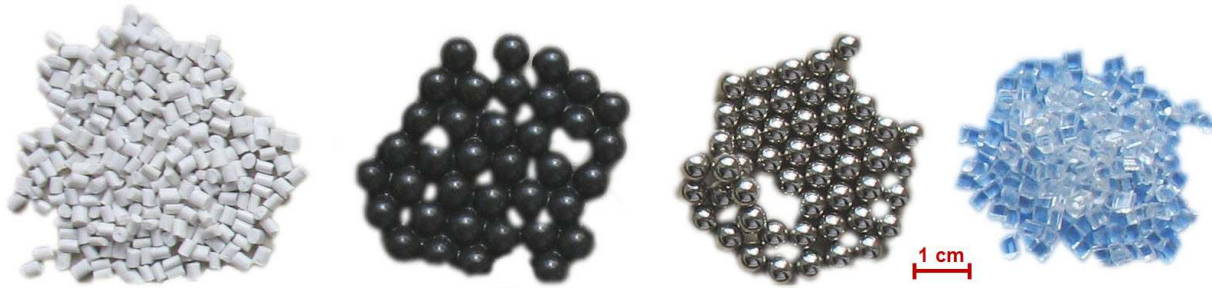
Figure 4.7: Types of the tested granular materials, from the left: plastic rollers, plastic spheres, steel spheres and plastic cubes.
