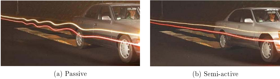
Figure 1.2: Comparison of the vertical displacement of a car with different types of suspension passing a road bump.
