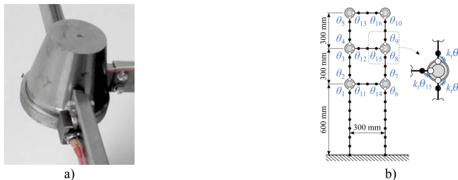
Fig. 1. a) Semi-actively lockable joint with visible beam-joint connections of the laboratory-scale frame structure and b) mesh of FE model with its dimensions and parametrization of each beam-joint connection.
