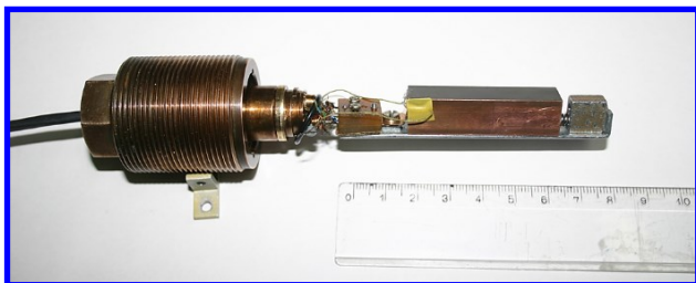
Fig.7. Love wave waveguide (on the right) consisting of an elastic surface layer (Cu) deposited on an elastic substrate (steel).
