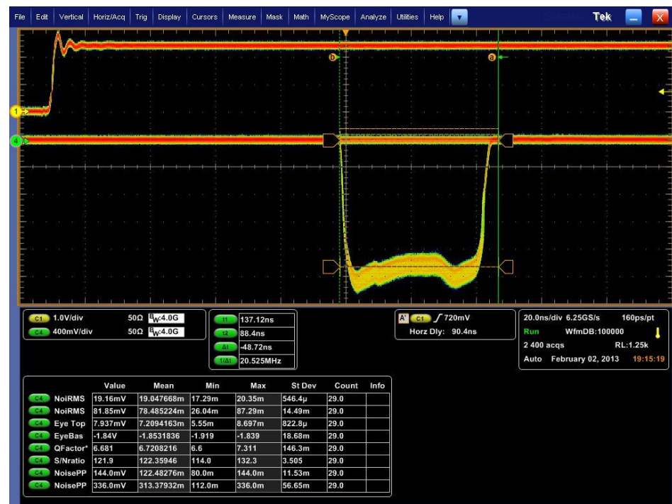
Figure 6. Sample oscillogram obtained during bit error rate (BER) measurements.
