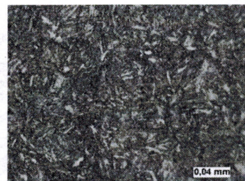
Fig. 6. Microstructure of high-tempered martensite in sample No. 3
