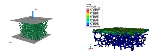
Figure 1: Numerical model for rigid mass impact testing of open-cell 96% porosity convex foam (left) and the equivalent plastic strain distribution for rigid plate impact with  $V_0$ =300 m/s and t=5.0  $\mu$ s (right).
