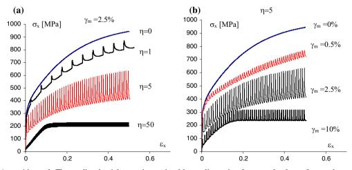
Fig. 18 Austenitic steel: The predicted axial extension assisted by cyclic torsion for several values of  $\gamma_m$  and  $\eta$ : a constant shear strain amplitude  $\gamma_m = 2.5\%$ , varying  $\eta = 0, 1, 5, 50$ ; b constant strain rate ratio  $\eta = 5$ , varying shear strain amplitude  $\gamma_m = 0\%, 0.5, 2.5, 10\%$ ;
