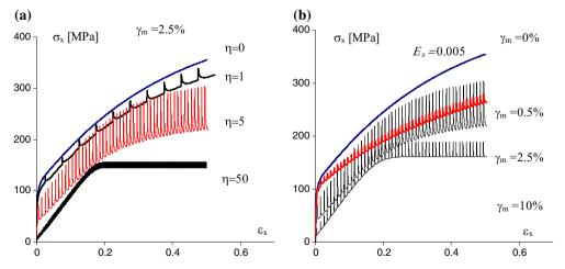
Fig. 11 Comparison of the tensile stress paths for piecewise linear shear strain control for different values  $\eta$  and  $\gamma_m$  for pure copper;—prediction by three-surface model: **a** prediction for  $\gamma_m = 2.5\%$  and different values of  $\eta$ , **b** prediction for  $E_x = 0.005$  and different values of  $\gamma_m$
