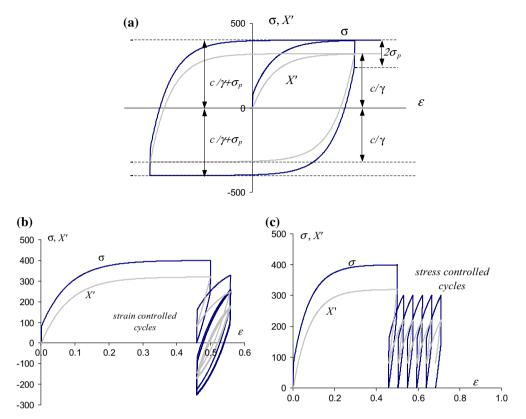
Fig. 3 Loading-unloading response in the uniaxial case; a symmetric strain controlled cycles; b strain controlled cycles after initial prestrain; c stress controlled cycles after initial prestrain
