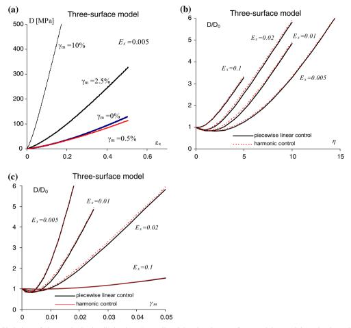
**Fig. 14** Variation of the total plastic dissipation D predicted by the three-surface model: **a** axial strain dependence for  $E_x = 0.005$ ,  $\gamma_m = 0, 0.5, 2.5, 10\%$  (or  $\eta = 0, 4, 2080$ ); **b** dependence of the ratio  $D/D_0$  on the strain rate ratio  $\eta$  for  $E_x = 0.005, 0.01, 0.02, 0.1$ ; **c** dependence of the ratio  $D/D_0$  on the shear strain amplitude  $\gamma_m$  for  $E_x = 0.005, 0.01, 0.02, 0.1$
