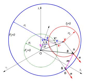
Fig. 6 Three-surface hardening model: evolution of the back stress Y toward the limit point  $Y_I$
