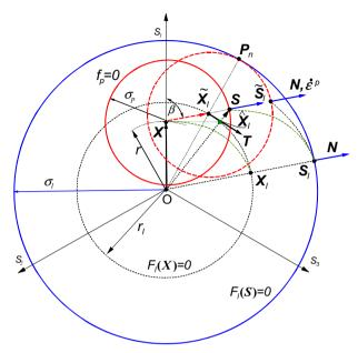
**Fig. 2** Evolution of the back stress X to its limit value  $\tilde{X}_l$  following Prager translation rule and subsequent reorientation process to the coaxial state  $X_l$
