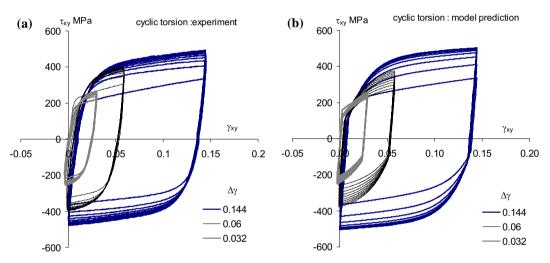
Fig. 17 Austenitic steel: cyclic torsion response for three values of shear amplitudes  $\Delta \gamma_{xy} = 0.032, 0.06, 0.144$ , a experimental data after Pawlicki and Grosman [65], b model prediction
