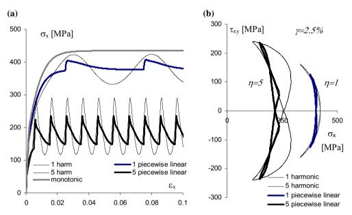
Fig. 13 Axial extension assisted by cyclic torsion for  $\eta = 0, 1, 5, \gamma_m = 0.025$  and saturated isotropic hardening; **a** axial stress evolution, **b** stress paths in the  $\sigma_x - \tau_{xy}$  plane
