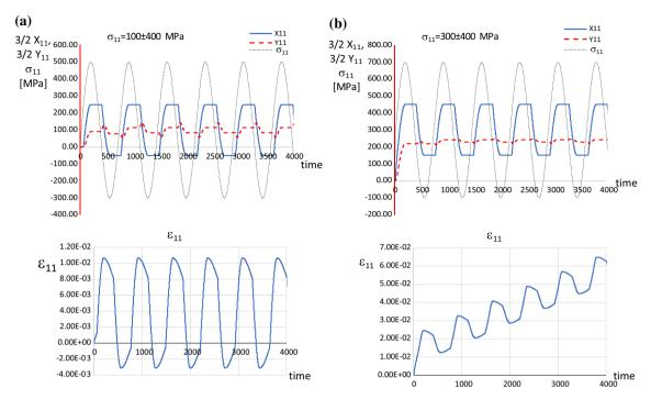
Fig. 7 Stress  $\sigma_{11}$ , backstress  $X_{11}$ ,  $Y_{11}$  and –strain  $\varepsilon_{11}$  response in the cyclic tension-compression for the three-surface model; a  $\sigma_{11} = 100 \pm 400$  MPa, b  $\sigma_{11} = 300 \pm 400$  MPa
