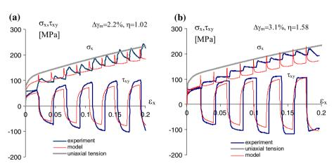
Fig. 15 Comparison of the three-surface model prediction with experimental data for axial extension assisted by cyclic torsion of pure copper for various  $\eta$ : **a** axial and shear stress evolution for  $\eta = 1.02$ ,  $\gamma_m = 2.2\%$ , **b** axial and shear stress evolution for  $\eta = 1.58$ ,  $\gamma_m = 3.1\%$
