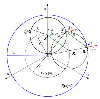
**Fig. 1** Evolution of the back stress X to its saturation value  $X_l$
