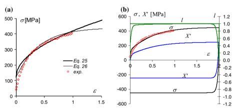
Fig. 4 Annealed copper: a Evolution of the limit stress  $\sigma_l$ , b the stress-strain curve for monotonic and reverse straining with the evolution of back stress and distance parameter l
