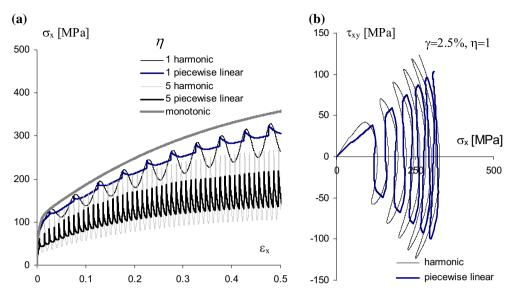
Fig. 12 Axial response for piecewise—linear and harmonic shear strain control for  $\eta = 0, 1, 5$  and  $\gamma_m = 0.025$ ; a axial stress evolution, b stress paths in the  $\sigma_X - \tau_{XY}$  plane
