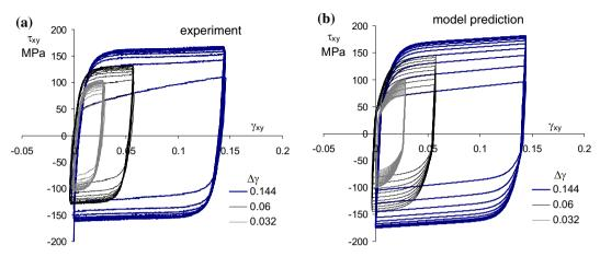
Fig. 9 Cyclic torsion response for three values of shear amplitudes  $\Delta \gamma_{xy} = 0.032, 0.06, 0.144$ , a experimental data, b three-surface model prediction
