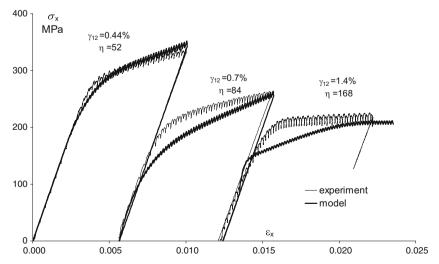
Fig. 16 Comparison of the three-surface model prediction with experimental data for axial extension with cyclic torsion of 2024 aluminum alloy for various process parameters:  $\gamma_m = 0.44 \%$ ,  $\eta = 52$ ;  $\gamma_m = 0.7 \%$ ,  $\eta = 84$  and  $\gamma_m = 1.4 \%$ ,  $\eta = 168$
