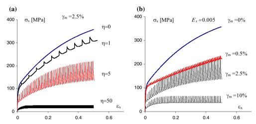
Fig. 10 Comparison of the tensile stress paths for piecewise linear shear strain control for different values  $\eta$  and  $\gamma_m$  for pure copper;—prediction by two-surface model: **a** prediction for  $\gamma_m = 2.5\%$  and different values of  $\eta$ , **b** prediction for  $E_x = 0.005$  and different values of  $\gamma_m$
