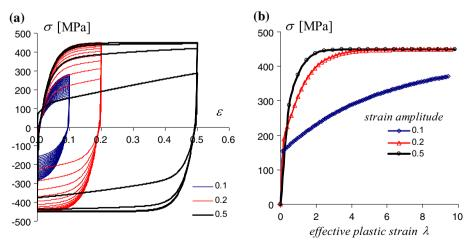
Fig. 5 Stress-strain response in the cyclic tension-compression test for various amplitudes: a evolution to steady states for specified amplitudes  $\varepsilon_a = 0.1, 0.2, 0.5$ , b evolution of the maximal stress in cyclic hardening process
