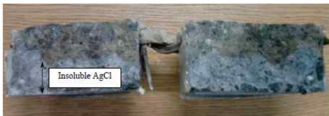
Figure 1: Section view of concrete specimen split after the chloride migration test and after spraying the surface with \text{AgNO}_3 solution
