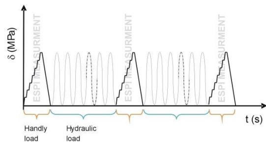
**Fig. 1** Diagram presenting sample load in fatigue cycles
