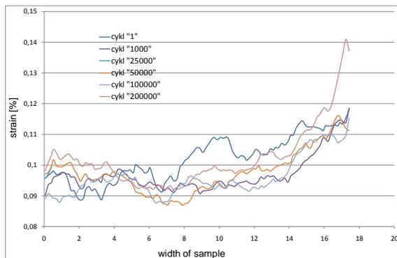
**Fig. 3** Lateral profiles of strain changes in the cross-section with the maximum values.
