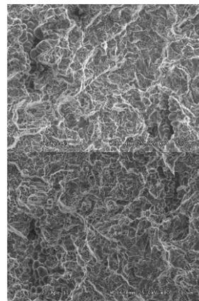
**Fig. 5** Some of the numerous pores on the fracture surface
