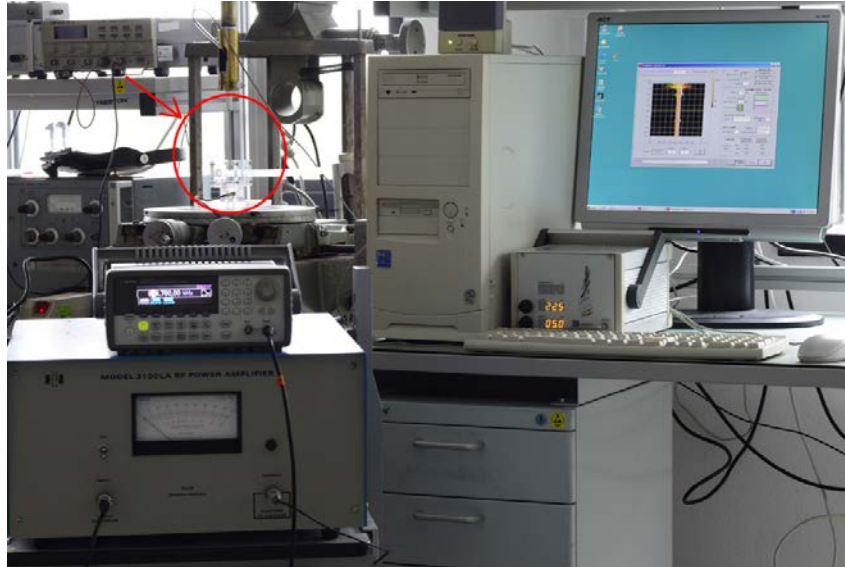
Fig. 3. Streaming measurement setup with the 20 MHz Doppler flowmeter connected to PC, using the GASP software (right). In the red circle, the 2 mm 20 MHz Doppler transducer was on top, silicone tube from Fig.6b was in the center (vessel removed), and 25 mm 1 MHz streaming generating transducer was at the bottom. The ENI 3100LA power amplifier and 33250A arbitrary function generator were on the left.
