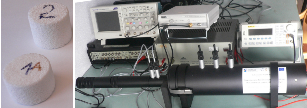
Figure 2: Two samples of ceramic foam \text{Al}_2\text{O}_3 with porosity 90% (left), and the impedance-tube experimental set (right).
