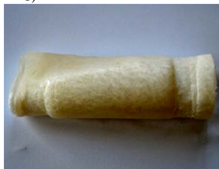
Fig. 2. The LV phantoms: a) – normal, b) with stiffened wall imitating the myocardial infarction.
