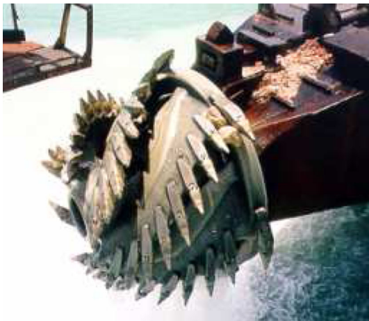
Fig. 1 Dredge cutter head
