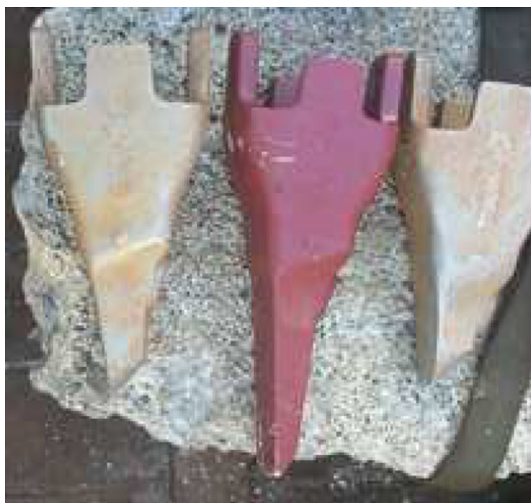
Fig. 3 Wear of rock cutting tools—new and worn dredger picks
