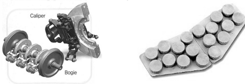
Figure. 1. Brake system for high speed train and sintered brake pads ( source: www.gobizkorea.com ).
