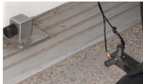
Fig. 5. Vibration transducers placed on the train floor.
