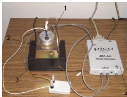
Fig. 1. The main elements of the measuring setup: 1 – chamber, 2 – electronic module, 3 – power supply, 4 – A/D converter.
